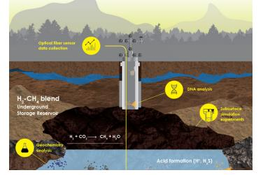
Underground storage of H<sub>a</sub> is less costly than storage in above-ground vessels but significant technical challenges must be addressed to store H<sub>2</sub> economically and safely at the commercial scale. SHASTA research focuses on quantifying materials compatibility, investigating core- and reservoir-scale performance and characterizing microbial interactions.
