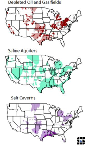
Three main types of underground natural gas strorage (USG) in service are: depleted oil and gas fields, saline aquifers, and salt caverns.
