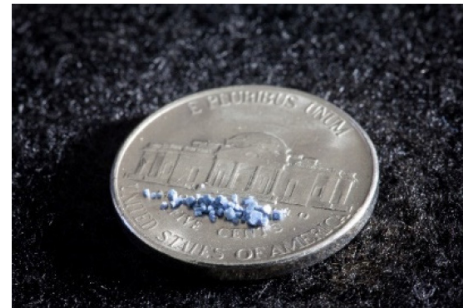
Figure 2. Metal organic framework materials have small porous holes that can selectively adsorb CO 2 over other gases.
