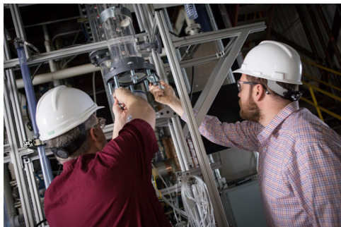
Figure 7. Researchers assembling the cold-flow carbon stripper.
