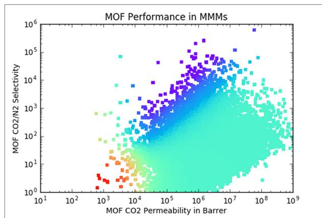
Calculated selectivity versus CO<sub>2</sub> permeability for a large database of MOF materials. Each point is colored based on the relative cost of carbon capture predicted for a hypothetical mixed matrix membrane made using that MOF. Cost is highest for red, moderately high for green, moderately low for blue and low for purple.
