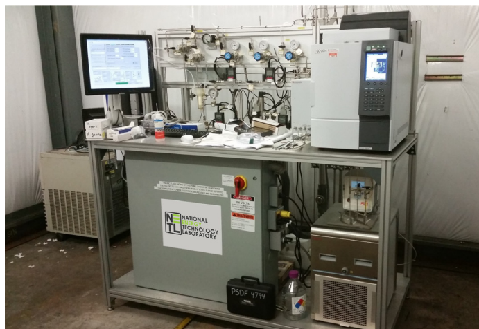
A test apparatus designed and built by NETL to measure gas permeance for CO 2 separation membranes at the National Carbon Capture Center in Wilsonville, Alabama.
