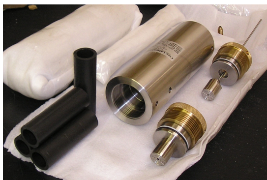
Figure 10. PPAL coreholder components.
