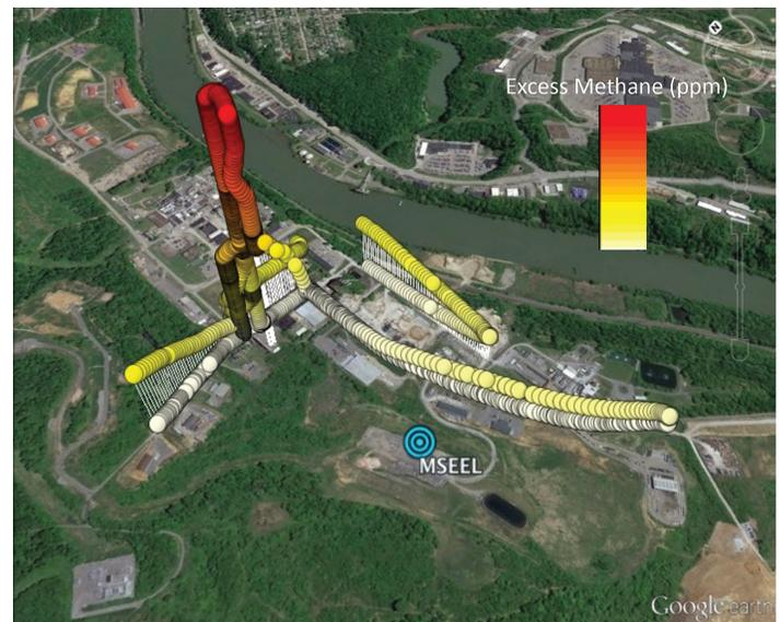
Results of a methane survey conducted during flowback operations at the Marcellus Shale Energy Environmental Laboratory (MSEEL), an active shale gas development site in Morgantown, West Virginia. High methane concentrations were observed downwind of the well pad. Data were used to estimate methane emission rate.
