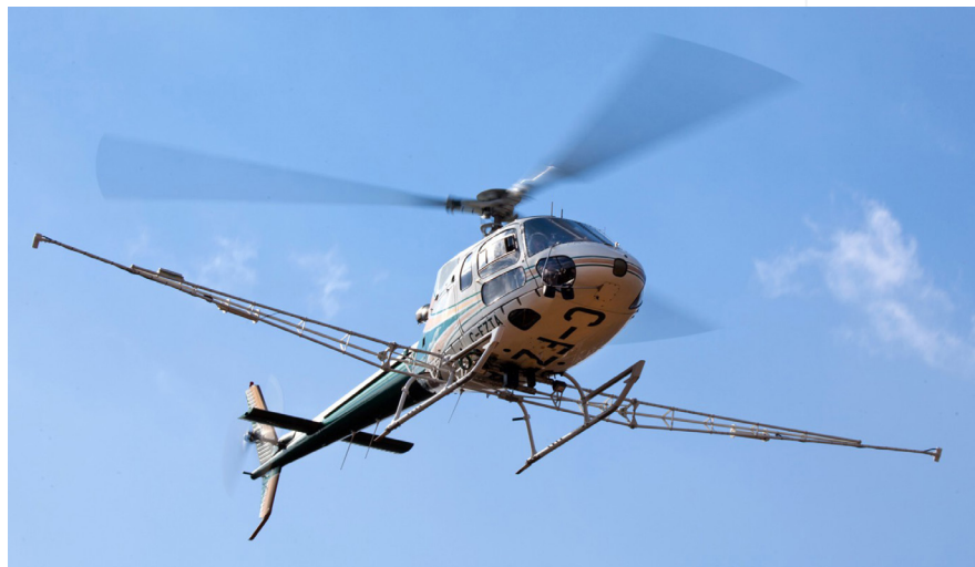
Helicopter with two, boom-mounted magnetometers surveying for existing wells at Marcellus Shale gas well location in Washington County, PA.
