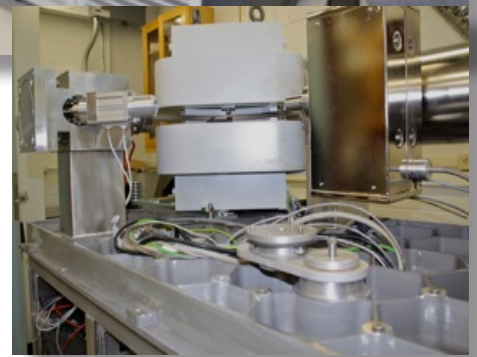
NETL's Multicollector ICP MS instrument, currently housed at the University of Pittsburgh, is used to measure isotope ratios in natural samples.
