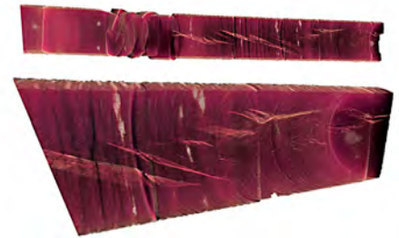
Two views of fractured Marcellus shale rock core colored to reflect mineral density.
