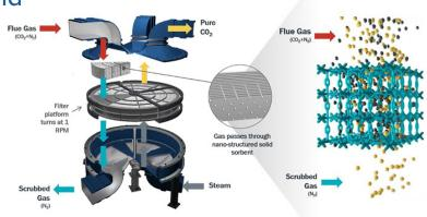
from flue gas streams and generates high-purity  $CO_2$  in about 60 seconds. Captured  $CO_2$  can then be stored permanently in the subsurface or reused as a feedstock for high-value chemicals and other applications.
