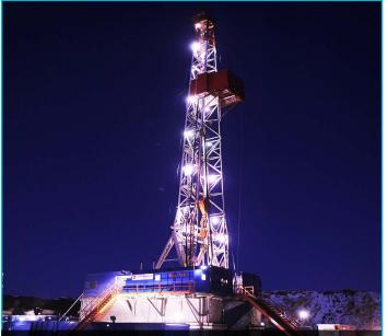
Rig drilling a site characterization well at the Craig Power Station in Colorado, USA. *Photo Source: Schlumberger Carbon Services*
