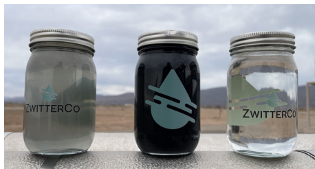
The left jar shows the wastewater stream sent through ZwitterCo's superfiltration membranes. The middle jar is the concentrate following membrane treatment. The right jar is the permeate from the membranes, enabling clean water for reuse.
