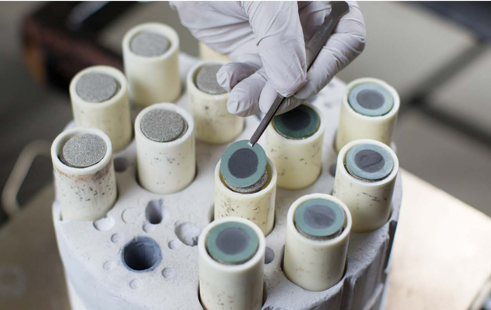
A researcher places SOFC button cells in NETL's multi-cell array testing platform for analysis.
