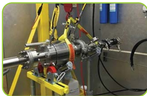
PCXT Chamber for Sub-Sampling and Transfer to Micro-CT
