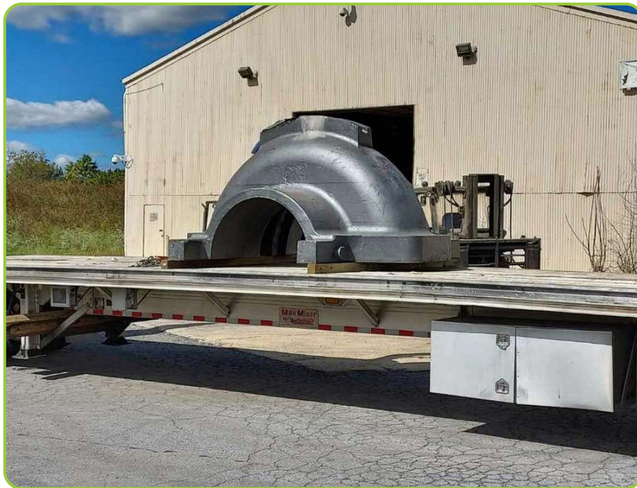
Actual H282 Casting Produced by the Project
