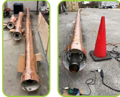
3- to 120-ft-Long Pipe-in-Pipe Set Up
