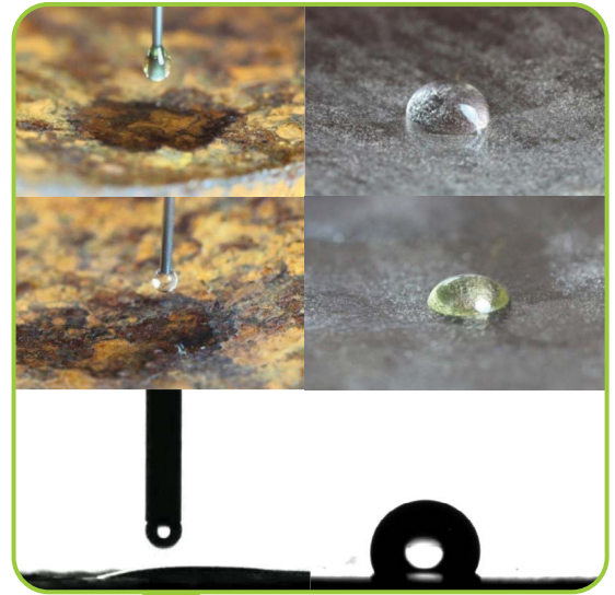
Image of Water Droplet on Untreated Pipeline (Left) vs. DragX™ Treated Pipeline (Right).
