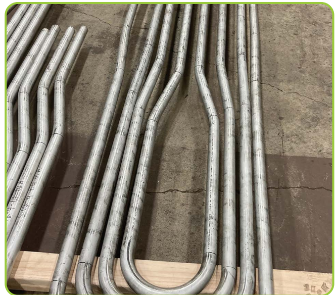
Haynes 282 Boiler Tube Assembly
