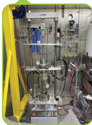
PCXT Anisotropic Permeability Chamber Measures Permeability in X, Y, and Z Directions
