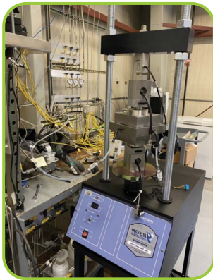
PCXT Anisotropic Permeability Chamber Measures Permeability in X, Y, and Z Directions
