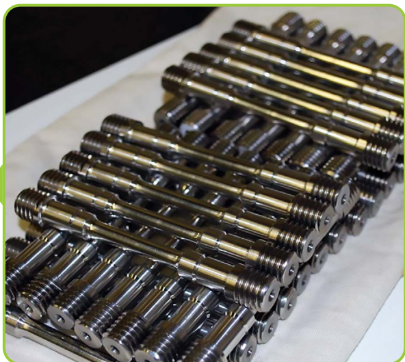
Haynes 282 Test Specimens
