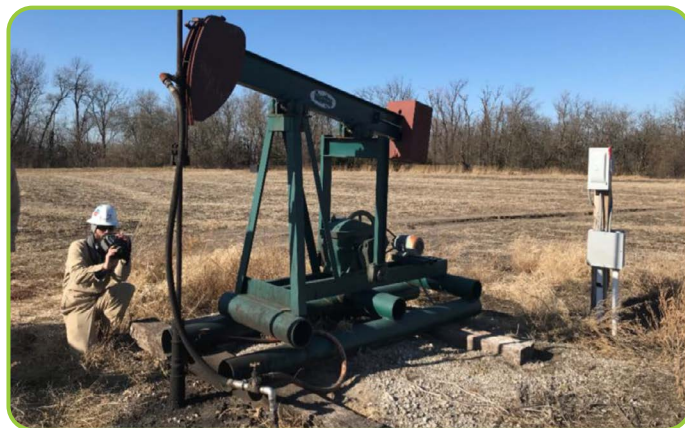
Emissions Were Identified Using an Optical Gas Imaging (OGI) Camera and Quantified, Where Possible, Using a Bacharach Hi-Flow Sampler (BHFS)
