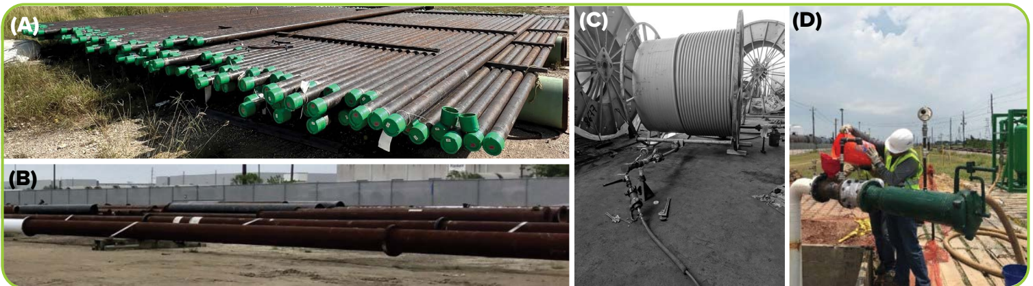
Test Applications of DragX™ Completed During This Effort Working With Different Industry Partners: (A) 8,000+ Feet of Casing Pipe, (B) 1,000+ Feet of Transport Pipe, (C) 10,000+ Feet of Coiled Tubing, (D) 1,000+ Feet of Wastewater Feed
