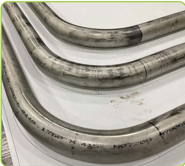
Haynes 282 Boiler Tubing
