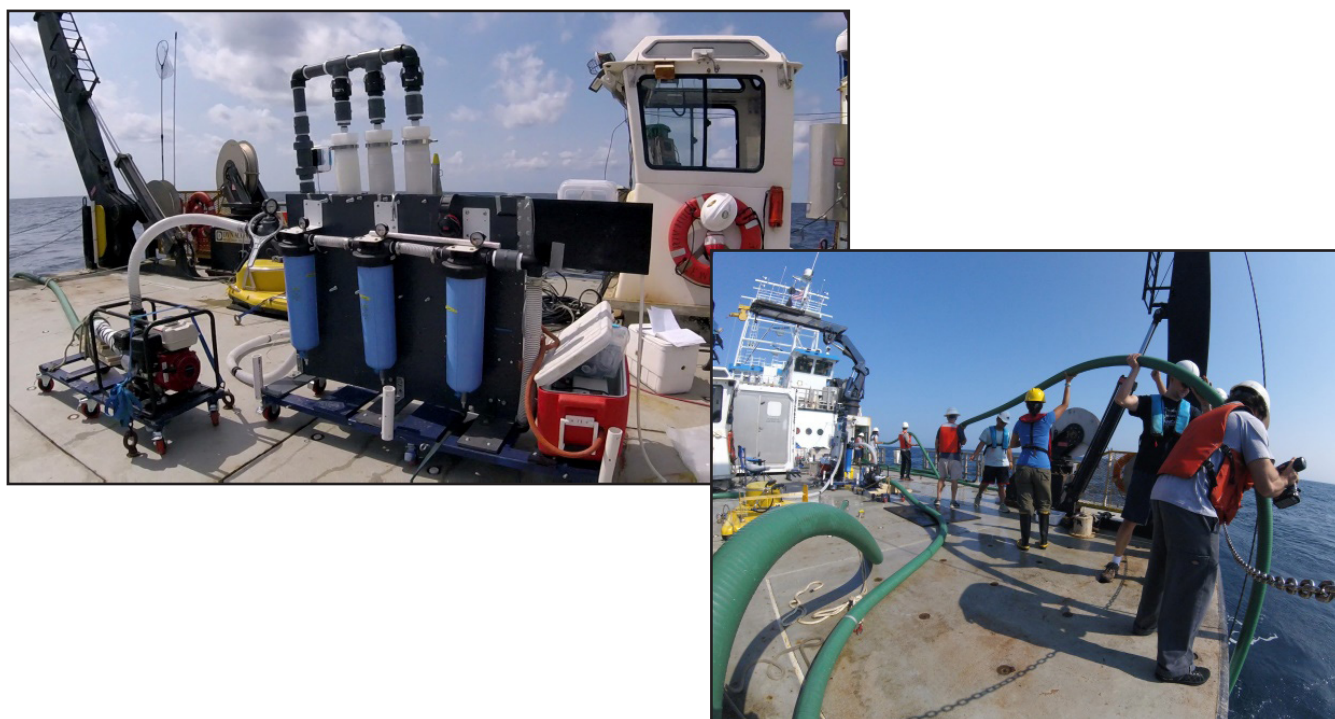
Figure 2. Equipment onboard the R/V Hugh R. Sharp, deployed on the U.S. Mid-Atlantic margin to sample and extract methane from seawater. Photos courtesy of USGS.
