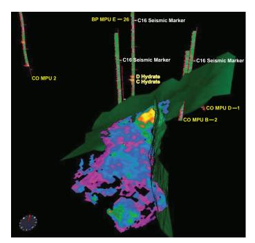
**Figure 2:** Milne Point—Mount Elbert gas hydrate prospect. Three-dimensional image of a fault-bounded, high amplitude feature (in a pallette of colors ranging from yellow to magenta; the yellow-imaged portion of the structure contains the thickest and most concentrated gas hydrate). Also shown are the bounding faults (in green) and gas hydrate occurrences in nearby well penetrations. The well penetrations show downhole-measured geophysical data indicative of gas hydrate occurrence (in yellow).
