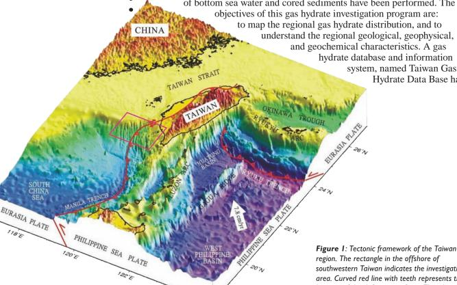
Figure 1: Tectonic framework of the Taiwan region. The rectangle in the offshore of southwestern Taiwan indicates the investigation area. Curved red line with teeth represents the location of the deformation front. The white arrow shows the direction and velocity of plate convergence.
