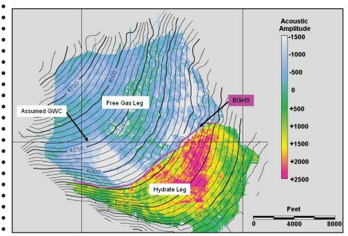
**Figure 3:** Time structure map of a possible hydrate saturated sand and downdip gas leg. The phase reversal across the BSR is illustrated on the amplitude overlay. Note that the downdip termination of the high negative amplitude conforms to structure fairly well.
