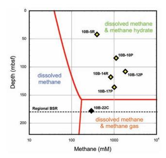
**Figure 6:** Methane concentration at a site in the Ulleung Basin, where gas hydrate was present as veins. Yellow diamonds indicate that IPTC measurements were made during depressurization.
