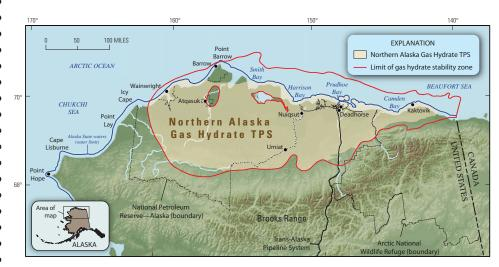
**Figure 1:** Map showing the Northern Alaska Gas Hydrate Total Petroleum System (TPS) (shaded in tan), and the limit of gas hydrate stability zone in northern Alaska (red outline).
