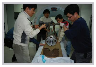
**Figure 1:** Scientists from KIGAM load a pressure core in a storage chamber onto the bed of the X-ray CT machine in Daejeon, Korea.
