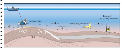
Figure 2: Schematic of survey equipment operation.
