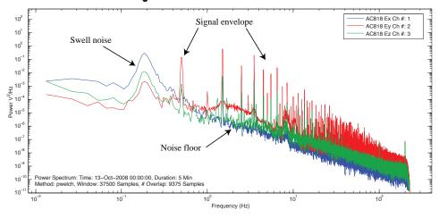
Figure 4: Spectrum of signals recorded on towed receiver Vulcan.
