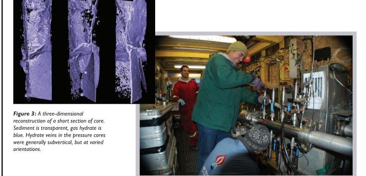
**Figure 4:** Carlos Santamarina and Tae Sup Yun making measurements on a pressure core using the IPTC.
