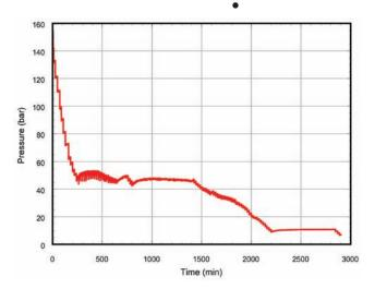
**Figure 5:** Depressurization curve for a core showing extended pressure "plateau" at hydrate stability boundary.
