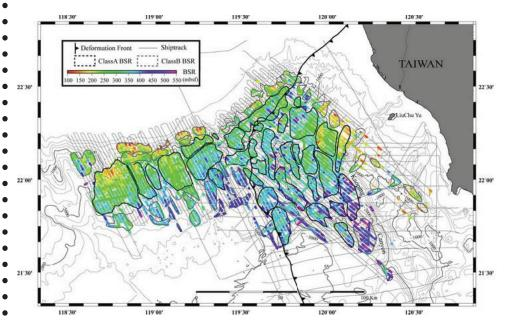
**Figure 2:** BSR distribution grouped by the quality of BSR appearance. Class A: clear and prominent BSR; Class B: possible BSR. Color indicates BSR sub-bottom depth. Curved black line with teeth represents the location of the deformation front which separates the convergent accretionary wedge province to the east from the passive South China Sea continental margin province to the west.
