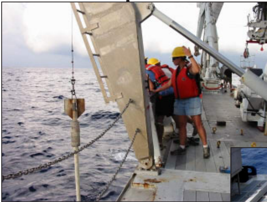
Graduate student Grace Castellini (Rice) gives hand signals to the crane operator during deployment of the gravity corer at the Bush Hill site.
