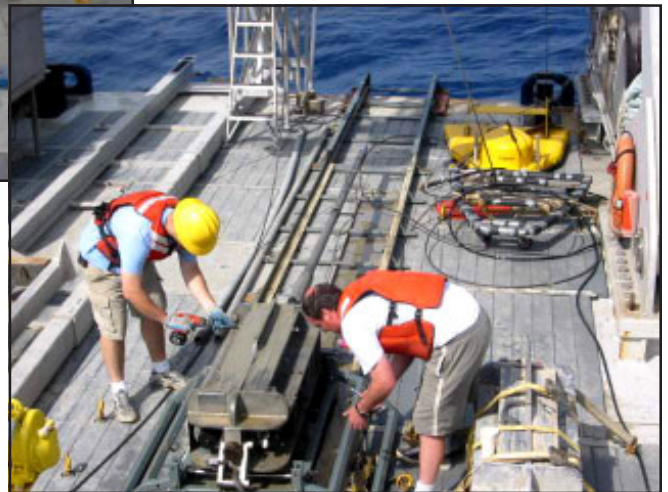
Heat flow technicians Chris LeBlanc and Walter Judge, both of Dalhousie University, service the short heat-flow instrument after recovery. The yellow instrument in the background is the Edgetech seismic fish used to obtain images of the shallow sub seafloor.
