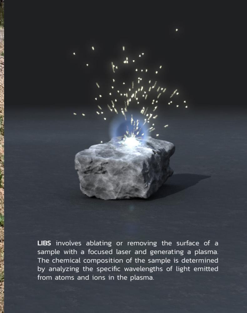
LIBS involves ablating or removing the surface of a sample with a focused laser and generating a plasma. The chemical composition of the sample is determined by analyzing the specific wavelengths of light emitted from atoms and ions in the plasma.
