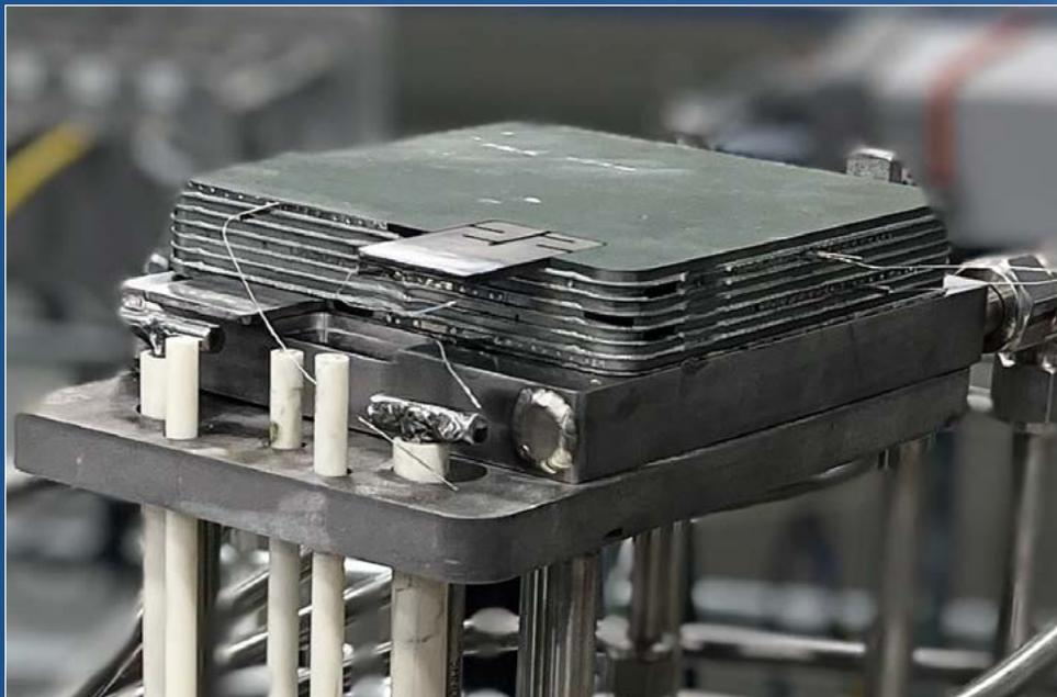
OxEon's solid oxide electrolysis cell.
