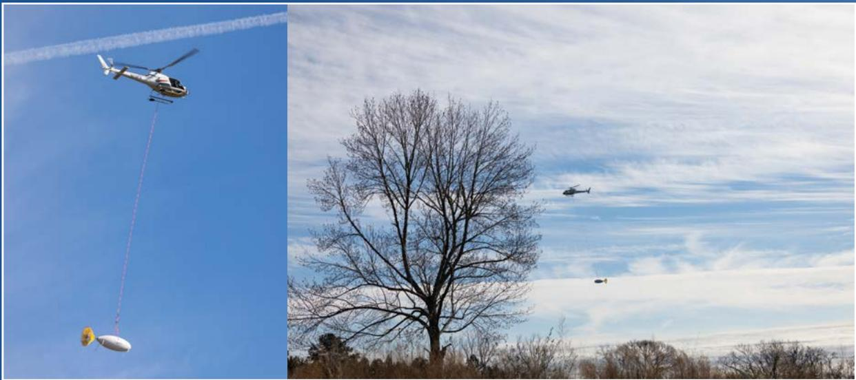
Airborne surveying of subsurface geologic storage site.
