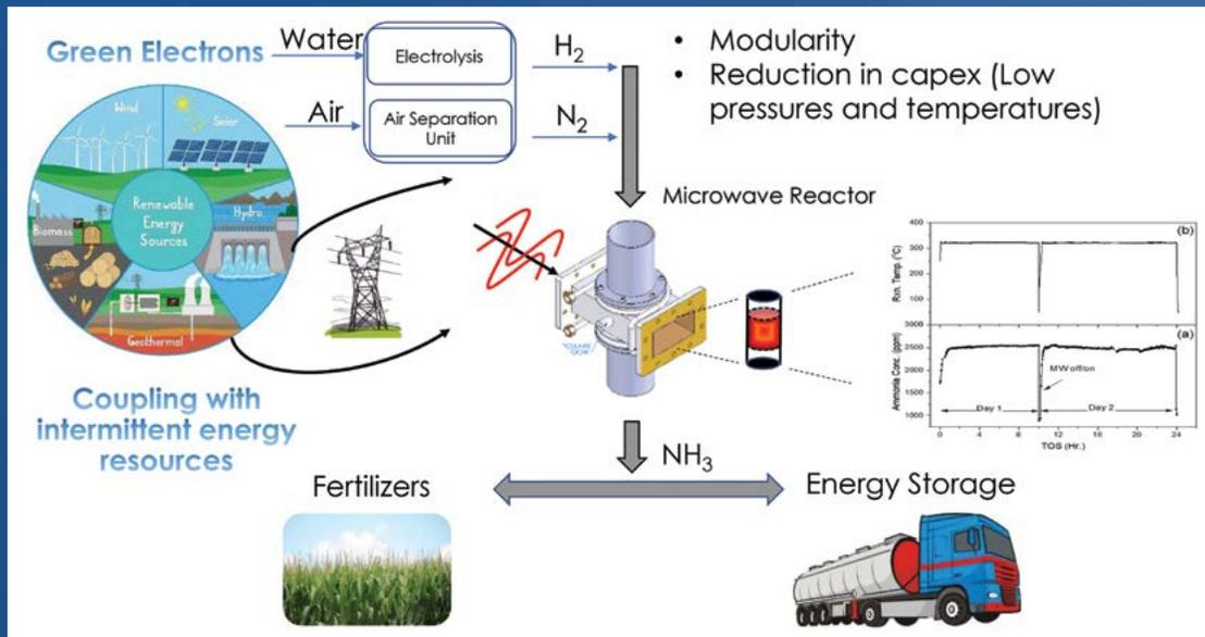
NETL ammonia (NH<sub>3</sub>) microwave process enabling point-of-use manufacturing.
