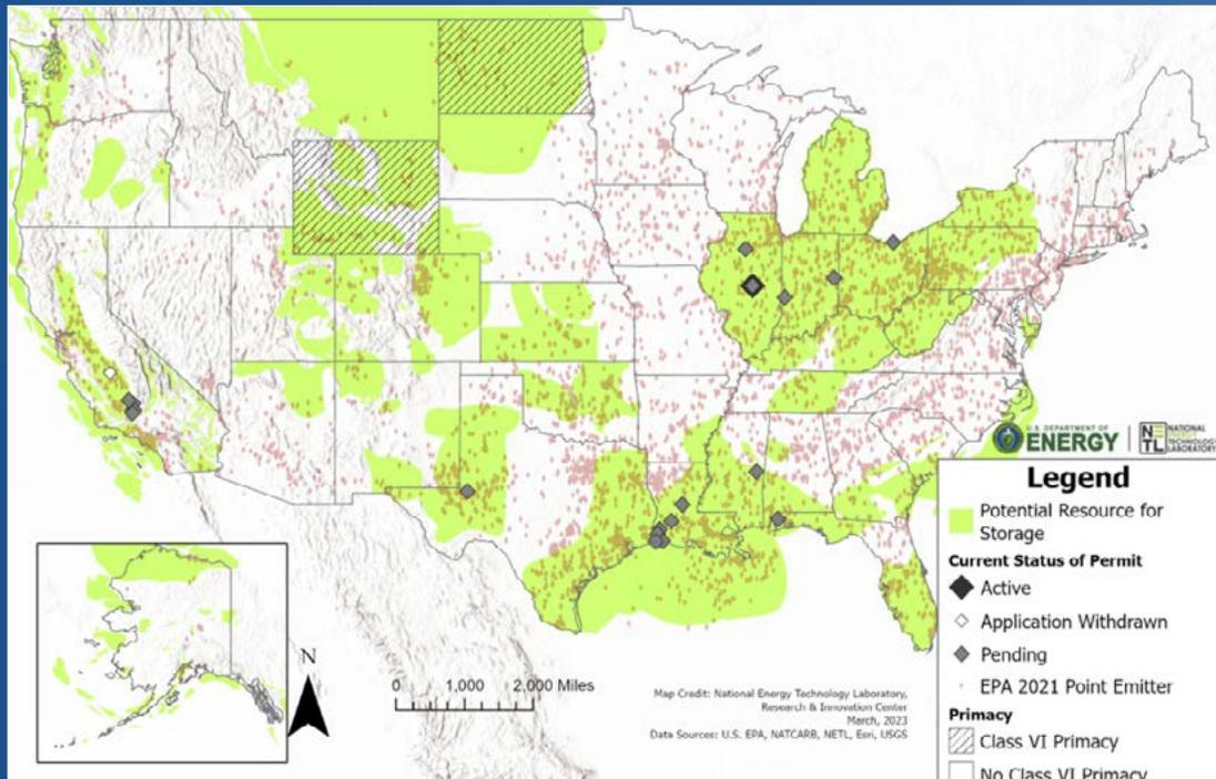
Class VI wells are used to inject carbon dioxide (CO<sub>2</sub>) into deep geologic formations for permanent storage. Permit applications require extensive data to ensure these wells are appropriately sited, constructed, tested, monitored, funded and closed.
