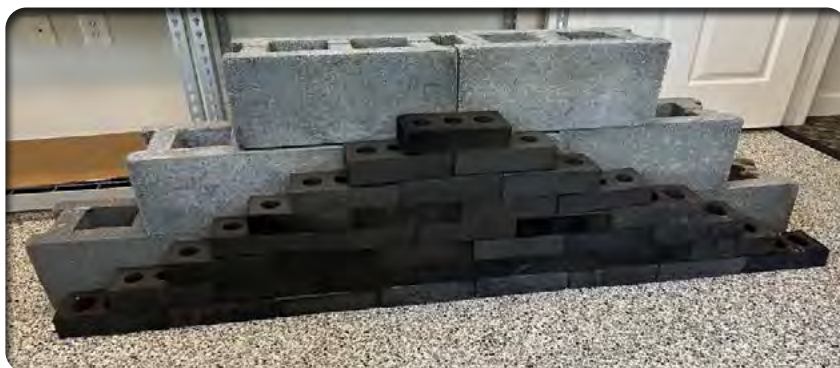
Coal-based bricks (X-BRIX) and blocks (X-BLOX).
