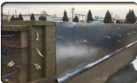
3-block, flue gas-heated testing modules.
