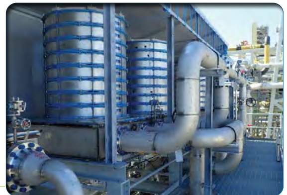
Planar module stacks with Gen-2 Polaris™ (2022 TCM field test).
