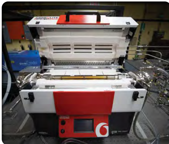
Inconel gas cell in a tube furnace enables high-temperature and high-pressure conditions to be replicated.
