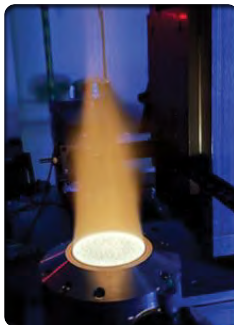
The combustion of a blend of a stoichiometric 50/50 mix of hydrogen/ammonia.
