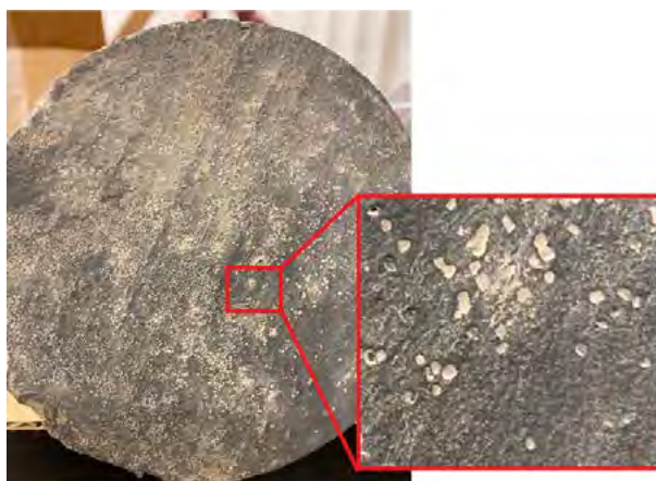
Proppant embedded in hydraulic fracture created through liner infill stimulation.
