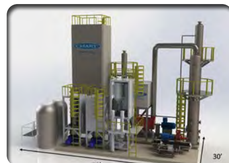
3-D model of a proposed site including the CCC skid.
