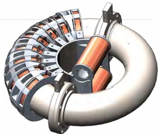
Tokamak magnet around hermetic housing for active magnetic regenerative cycle.
