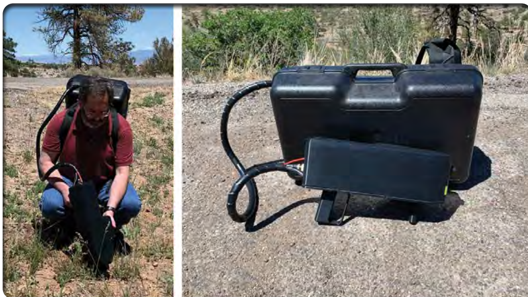
Left: The field-portable LIBS and Raman (backpack) prototype unit undergoing field testing. Right: Close-up of the field-portable unit.
