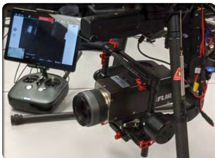
Left: Ronin Gimbal outfitted with an OGI camera; the Gimbal allows for controlled omnidirectional pointing of the camera
