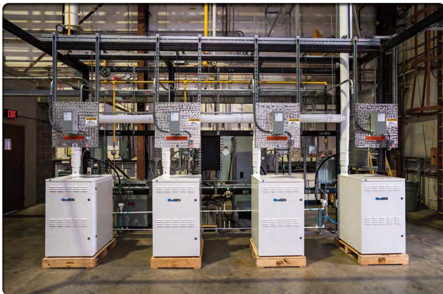
Four Aris SOFC stacks in the test stand at Morgantown.
