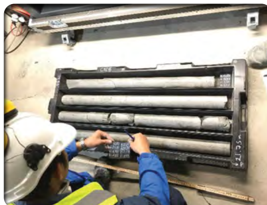
Drilling and coring at Mont Terri with 52mm ID casing.
