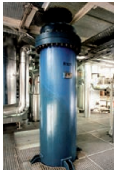
Figure 4: The TREMP™ semi-commercial reactor used for production of 200 Nm 3 /h of SNG product.
