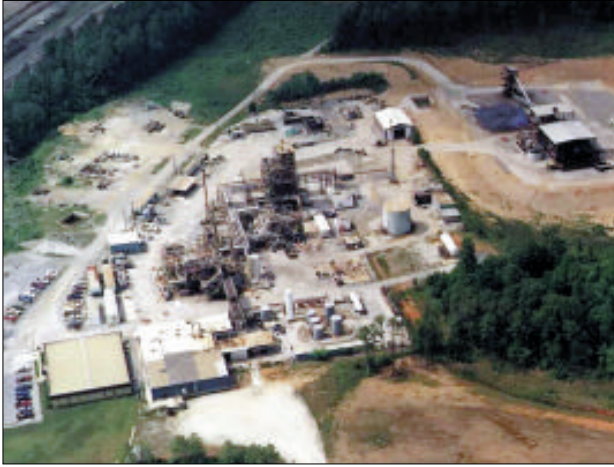
Figure 7. SRC-1 6 tons/day direct liquefaction plant at Wilsonville
