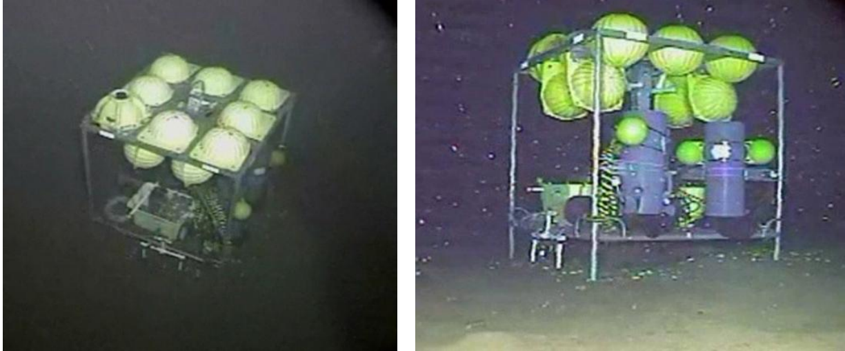
Figure 9. The ECOGIG lander, built by the MMRI/CMRET shop, was located 115m from the location given the navigation. Using the SSD's sonar and multiple camera capabilities, we were able to locate the lander, then survey its position, document the orientations of the instruments and remove the chimneys (grey cylinders in the front of the image on the right) and place them on the seafloor where the seafloor showed signs of gas emissions (bacterial mat, pitted surfaces).
