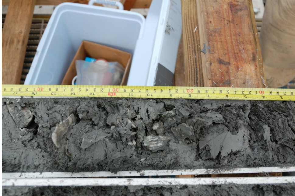
Figure 16. After 2 hours on deck, hydrate can still be observed in the bottom sections of JPC-001. The core contained hydrate layers, nodules, blades, grains and granules in extremely fine-grained host material.
