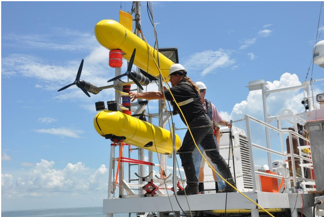
Figure 12. The AUV team prepares to launch the Mola Mola photo-AUV from the Pelican's upper deck.
