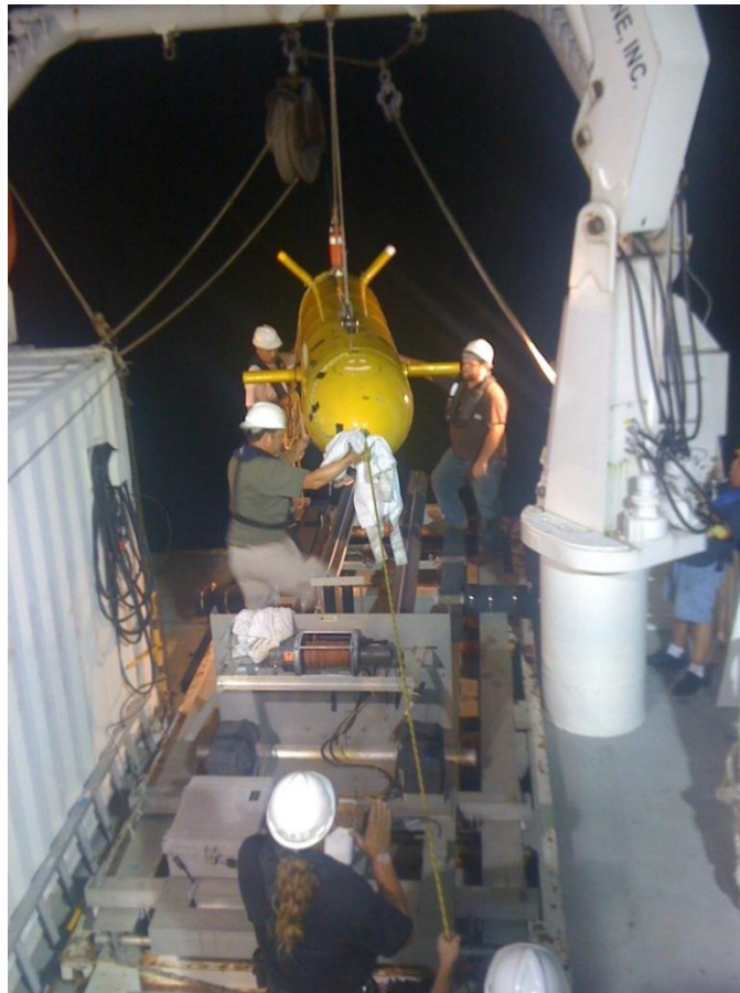
Figure 10. The AUV team prepares to launch the Eagle Ray AUV from the Pelican's maindeck via the launch and recovery system (LARS), designed and built specifically for it.
