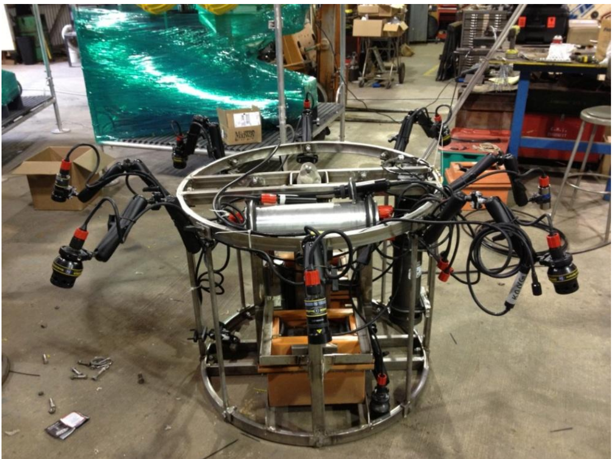
Figure 15. The Site Reconnaissance Camera, or SRC, designed and built at the MMRI shop – with input from researchers and assistance from the NIUST shop – will make its marine debut in March, 2013. Cameras, lights, and USBL navigation will provide the ability to “see” specific locations on the seafloor. The SRC will be used to verify and investigate seafloor features and instruments prior to coring, while deploying instruments, or making recoveries.
