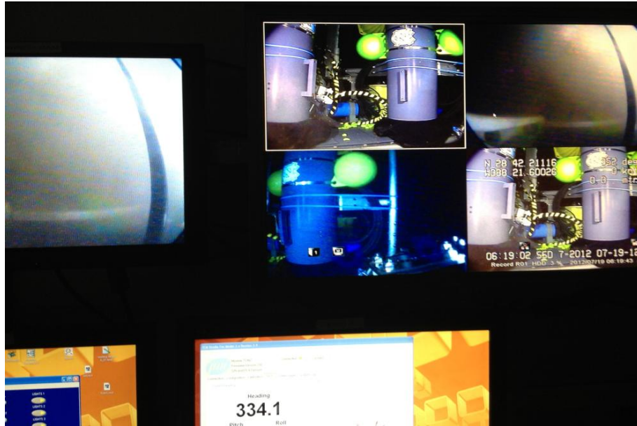
Figure A2. SSD operations monitor shows multiple cameras displayed in real time. All video is recorded for later examination, site verification, and study.
