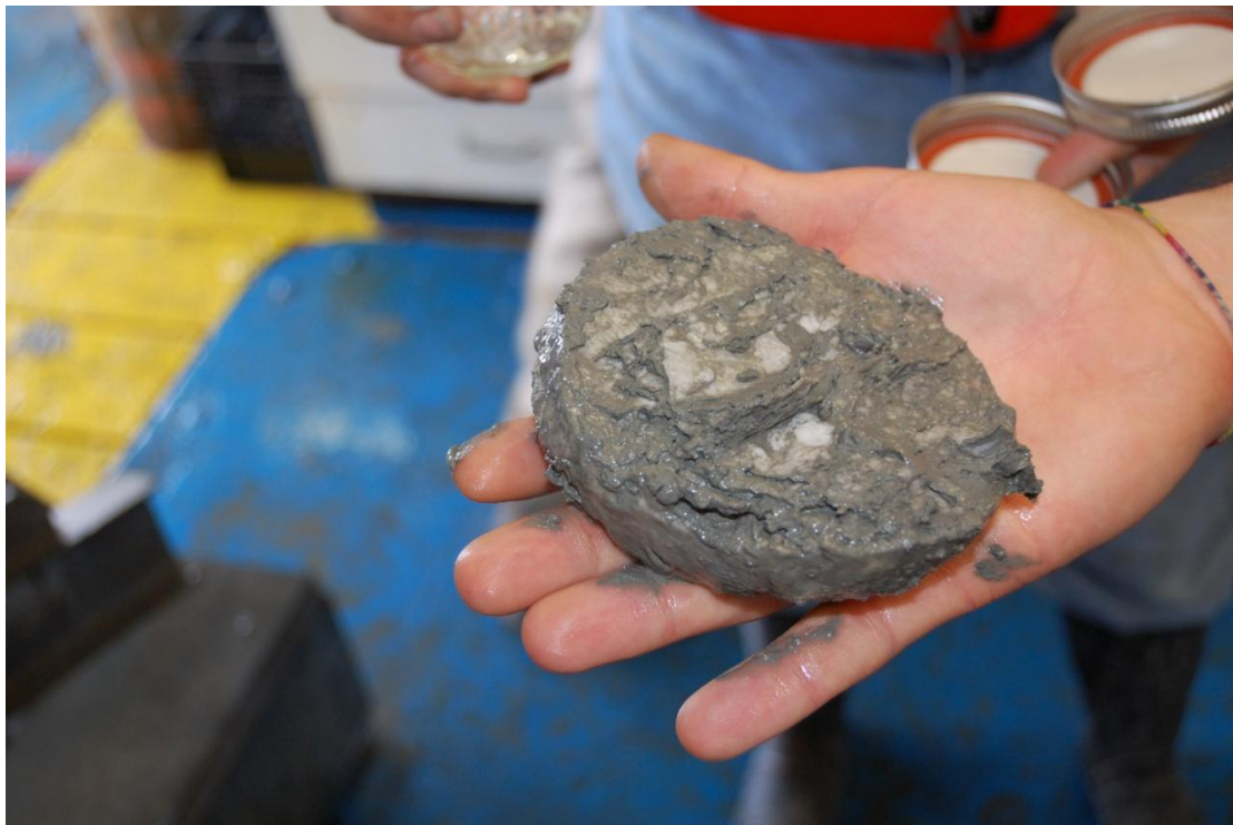
Figure 27. A disk of hydrates ~.8 in thick covered the entire cross-sectional area of JPC-001, 5.5 ft from the bottom of the core section.
