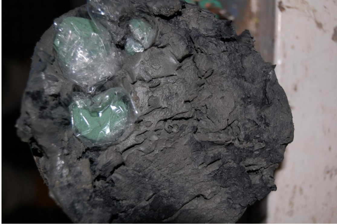
Figure 24. Sampled top of a section of JPC-006 shows high organic content and gas expansion.
