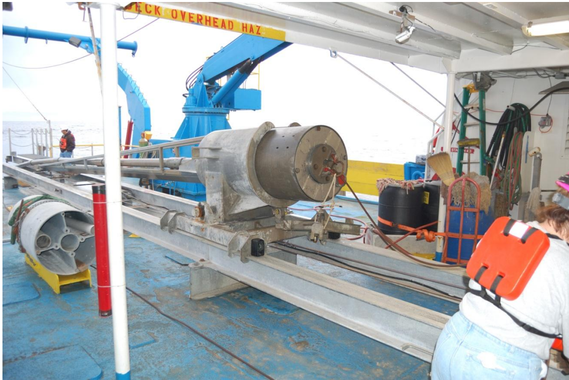
Figure 22. Recovery of the Jumbo Piston Corer to the deck.
