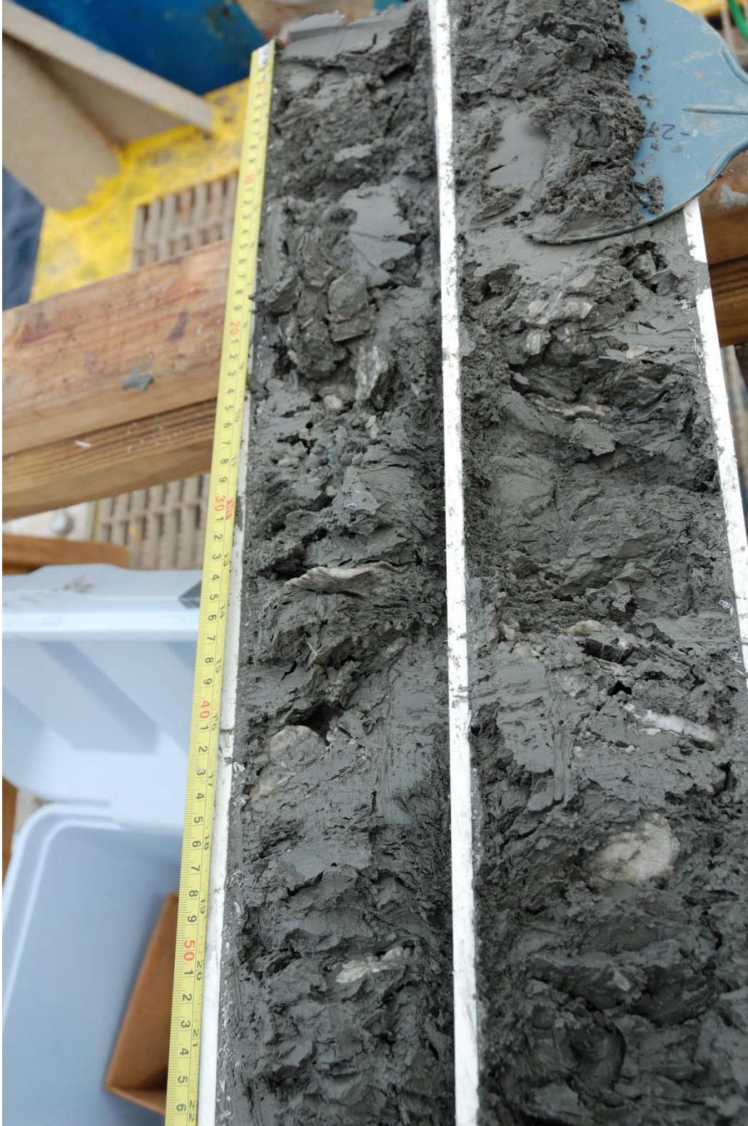
Figure 31. After 2 hours on deck, hydrate can still be observed in the bottom sections of JPC-001.
