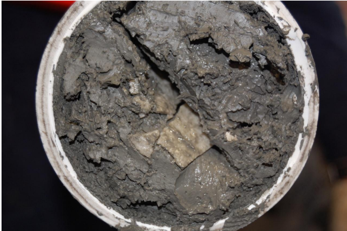
Figure 26. Chunks of hydrate 6 feet from the base of JPC-001.
