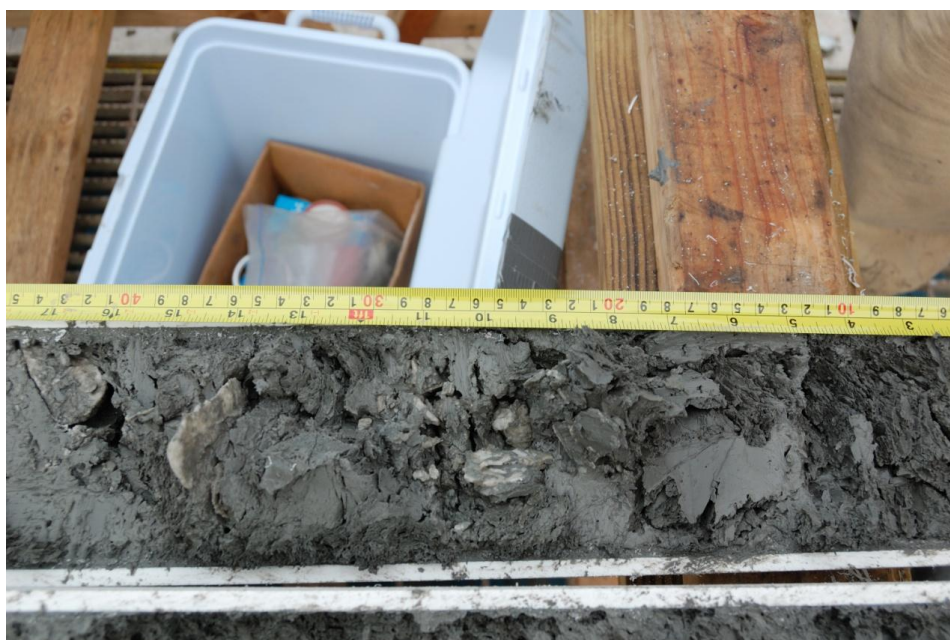
Figure 6. After 2 hours on deck, hydrate can still be observed in the bottom sections of JPC-001. The core contained hydrate layers, nodules, blades, grains and granules in extremely fine-grained host material.
