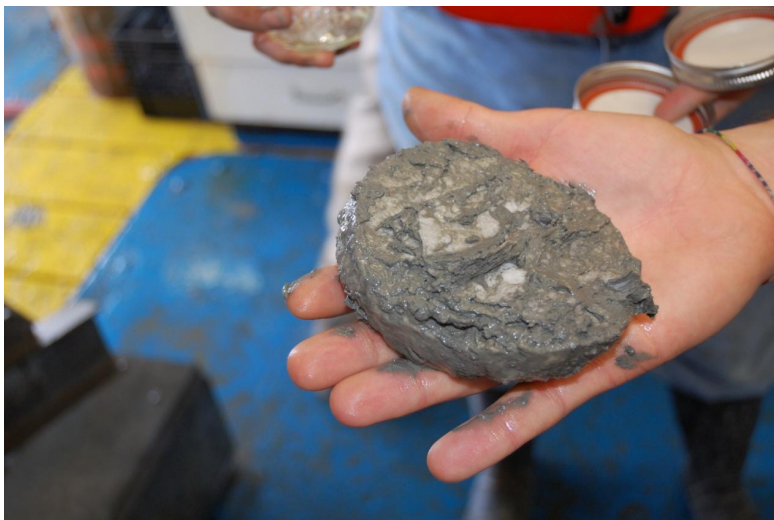
Figure 5. A disk of solid hydrate was recovered in the core barrel ~1m from the bottom of the core, JPC-001.
