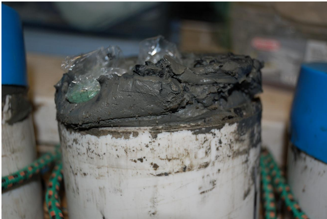
Figure 25. Top pf JPC-006; Note gas expansion, typical of JPC-006.
