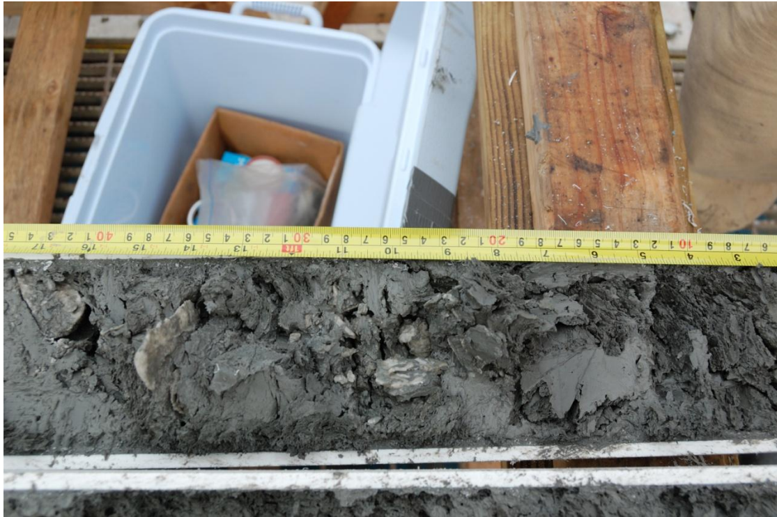
Figure 29. Bottom 3 ft section of JPC-001 contained hydrate nodules, blades, grains and granules.
