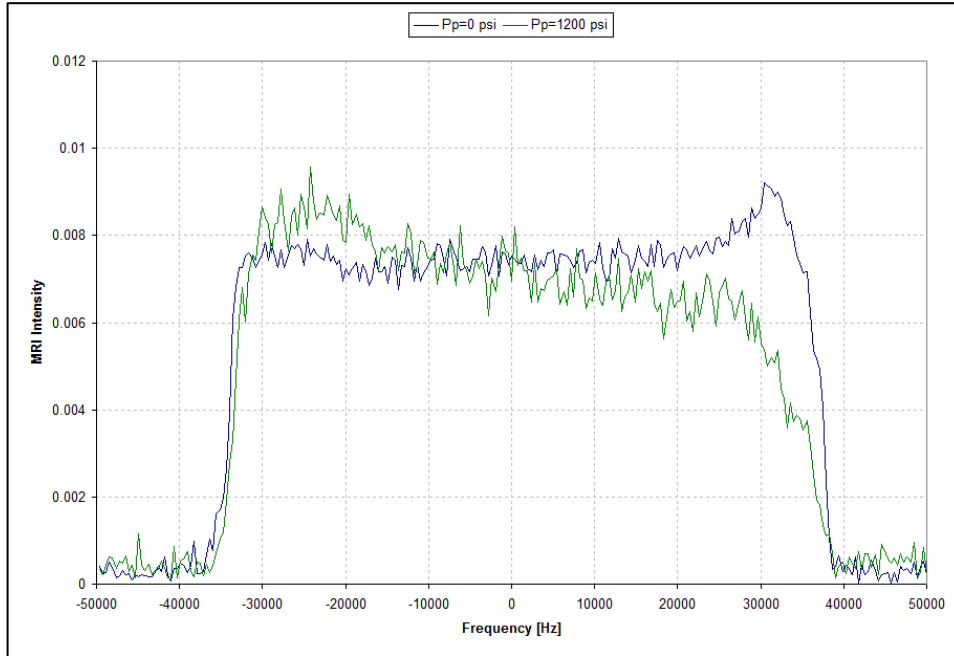
Figure 90: MRI profile along the longitudinal axis of the Bentheim sandstone core shows a uniform initial water saturation of 70% before hydrate formation.
