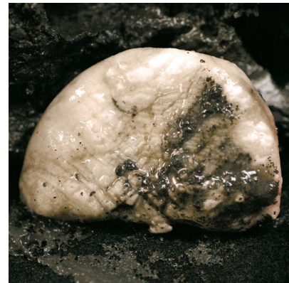
Figure 2.10: Gas hydrates in clay-rich sediments. Gas hydrates have been discovered in rich deposits characterized by dense arrays of nodules and hydrate-filled fractures in clay-rich sediments. Left: CT image of a core samples collected offshore India in 2006. The hydrate-filled veins appear as white (from a paper by Rees et al. 2011, published by JPGP, permission would be needed). Above pictures, gas hydrate samples (courtesy NGHP Expedition-01 science party).
