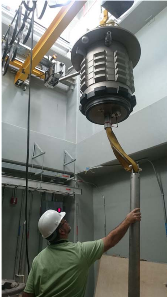
Figure 3: High pressure vessel and pressure test.
