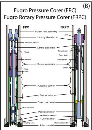
Figure 14. Diagrams of pressure core systems: (A) Pressure Core Sampler (PCS); (B) Fugro Pressure Corer (FPC) and Fugro Rotary Pressure Corer (FRPC).
