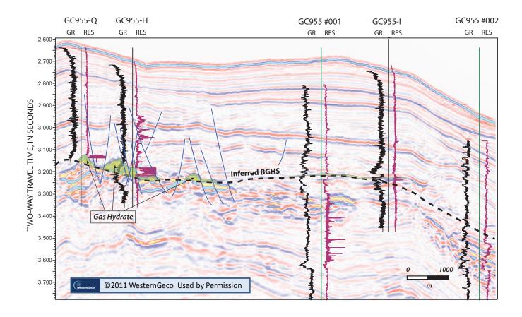
Figure 11. Logging while drilling data for three Gulf of Mexico JIP Leg II wells posted upon an arbitrary display of seismic data at the GC955 site. Green coloration shows the inferred methane hydrate occurrences at the base of methane hydrate stability (dashed line) (modified from Boswell et al., 2012a). Seismic data 2011 WesternGeco, used by permission.
