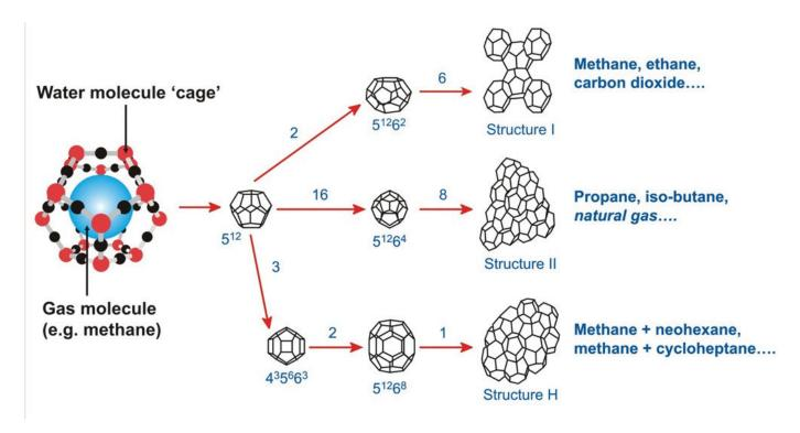
Figure MH 2. Hydrate crystal structures. The water cages that make-up the hydrate structures are depicted. Also shown are the three structure types that have been observed for hydrates: Structures I, II and H (modified from http://www.pet.hw.ac.uk/research/hydrates\_what.htm).
