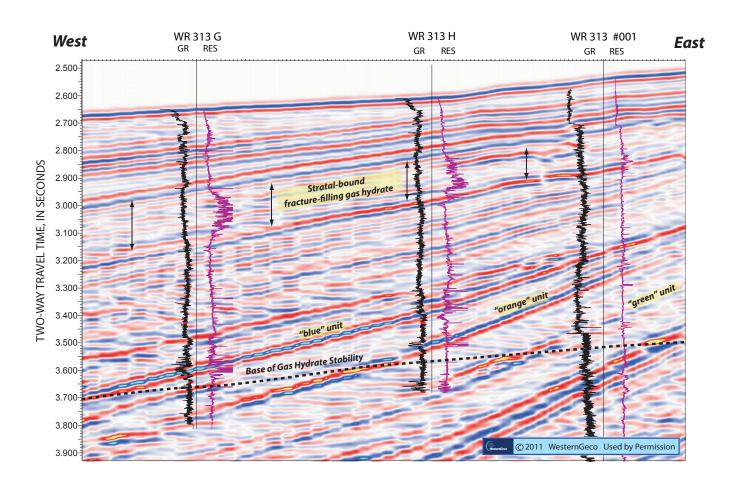
Figure 10. Overlay of select logging while drilling data from Gulf of Mexico JIP Leg II WR313-G and WR313-H wells on regional seismic data showing the major occurrences of methane hydrate, including a shallow, strata-bound zone interpreted to host methane-hydrate filled fractures in fine-grained sediments and deeper occurrences as pore-fill in sand (modified from Boswell et al., 2012a). Seismic data 2011 WesternGeco, used by permission.
