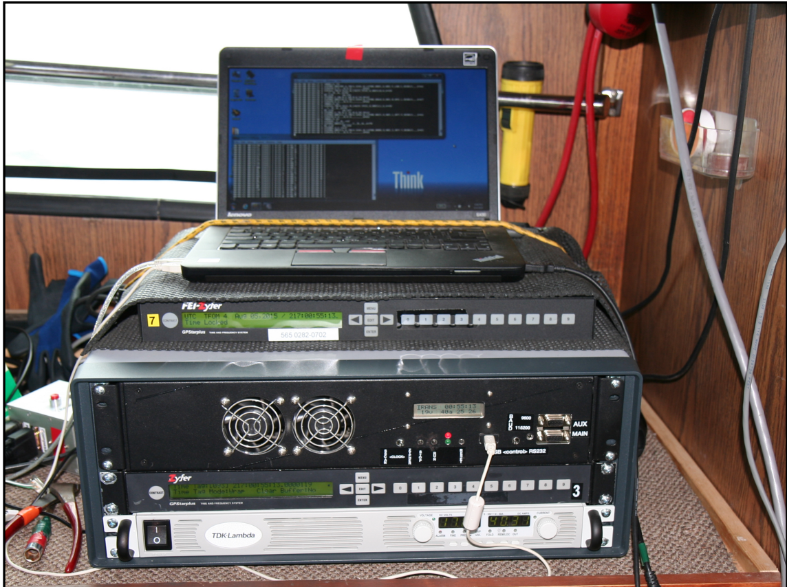
Figure 1: Compact transmitter, operates off 110VAC and capable of constant current output of up to 50 amps on a 50 meter antenna.
