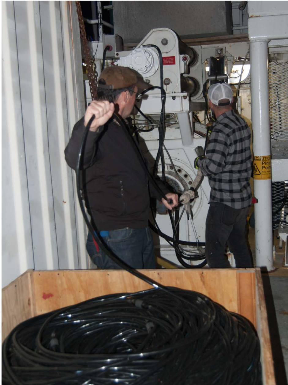
Figure 1. Spooling the 1100m Direct Current Resistivity Array onto the Pelican's Dynacon winch for deployment in survey/reconnaissance mode. Note nodes wrapped in grey tape.
