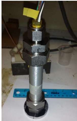
Figure 9: Aluminum pressure cell for use inside CT scanner
