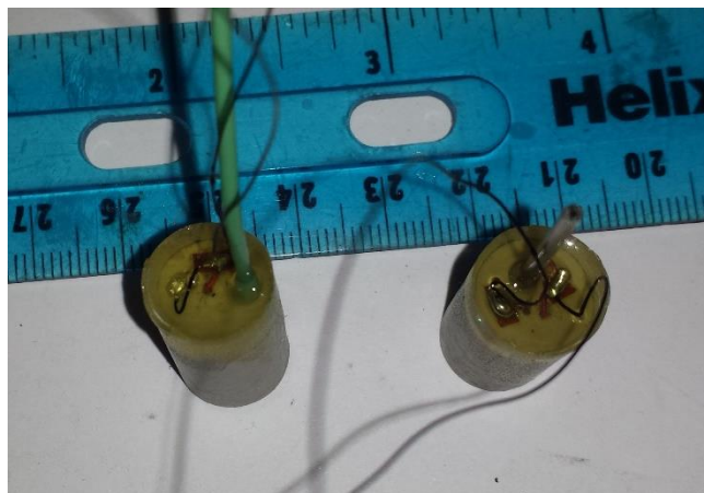
Figure 10: Ultrasonic P-wave transducers for use inside micro CT scanner.
