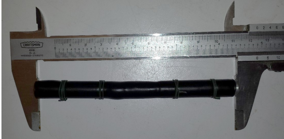
Figure 7: Sample jacketed in heat shrink tubing. The tested samples consisted of aluminum cylinders on both ends and quartz sand, sandstone or glass beads in between
