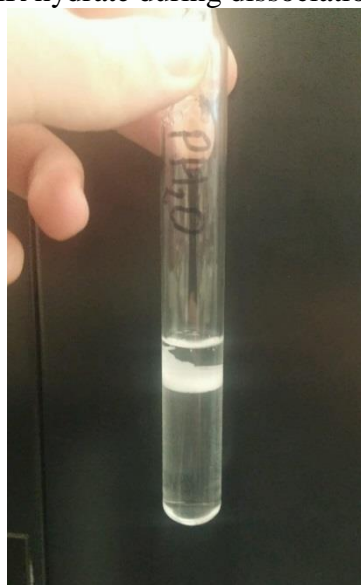
Figure 4: Partially dissociated cyclopentane hydrate. This stable condition is marked by the presence of an interface between two different fluids that might cause the late time responses in recorded NMR T2 spectra.
