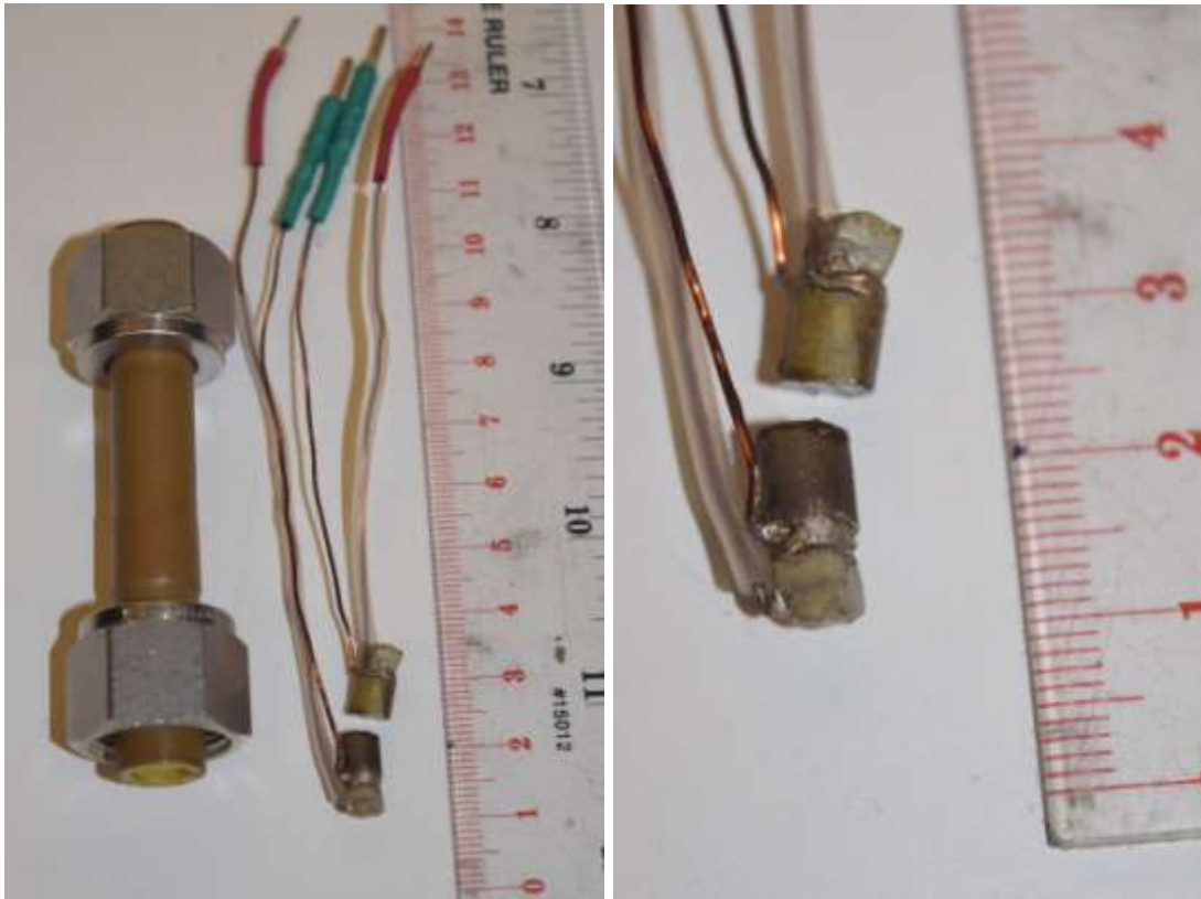
Figure 9. Ultrasonic P-wave transducers and torlon pressure vessel for use in MXCT scanner
