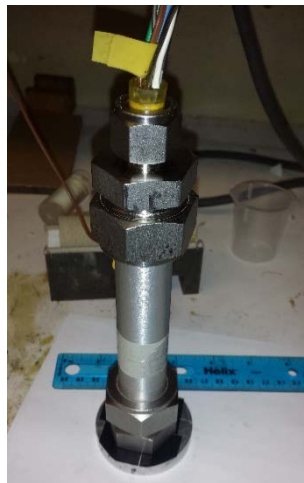
Figure 4: Aluminum pressure cell for use inside CT scanner
