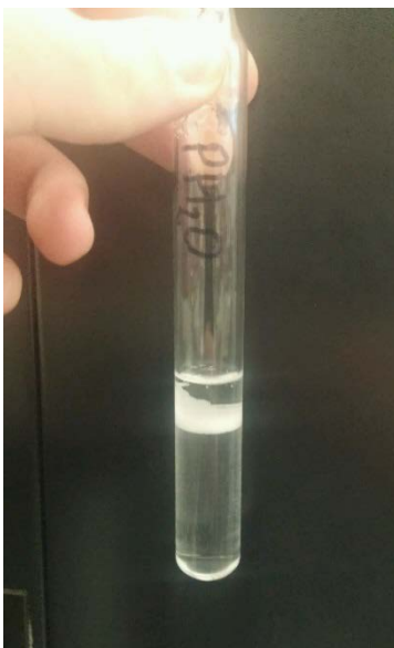
Figure 82: Partially dissociated cyclopentane hydrate. This stable condition is marked by the presence of an interface between two different fluids that might cause the late time responses in recorded NMR T2 spectra.
