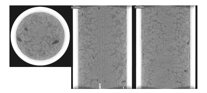
*Diatomaceous earth*: Hydrate forms around the periphery (irregular), and some lenses form in the center of the specimen. The fraction of segregated hydrate decreases with the increase in effective stress, i.e., specimen depth.
