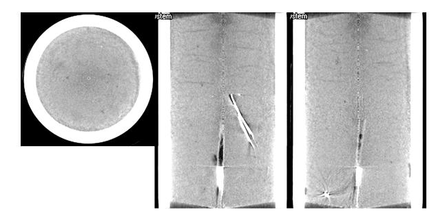
*Silica flour:* For comparison, solid silica flour particles are of the same size as porous diatom grains. Segregated hydrate is observed only at the top of the specimen. The duration of the thermal spike during phase transformation is much shorter in silica flour than in diatomaceous earth (possibly the effect of location relative to nucleation sites).
