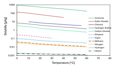
At standard pressure-temperature conditions, Argon, Krypton, Xenon, and Radon have higher solubility in water than that of methane gas. Other advantages of using noble gases as hydrate former include (1) high attenuation of X-ray intensity so that noble gas hydrate can be easily distinguished in CT images, and (2) much lower hydrate stability boundaries than that of methane and CO<sub>2</sub> hydrate.
