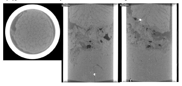
THF hydrate topology in different types of fine-grained sediments
