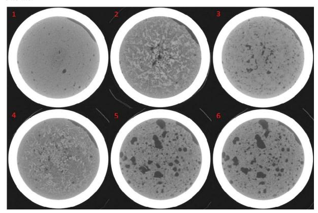
The X-ray image sequence above shows (1) the initial stage, (2) hydrate formation at 2°C (Note that the segregated bright parts are consolidated bentonite), (3) dissociated specimen, (4) hydrate and ice formation at -20°C, finally (5 and 6) show cross sections of the specimen one hour and one day after dissociation.
