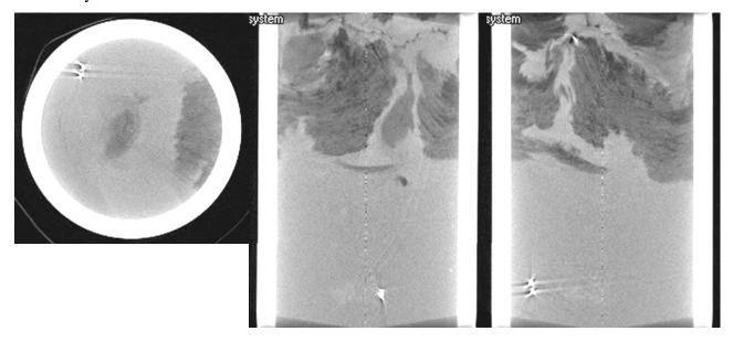
The X ray image after dissociation and re-formation cycle follows. The image on the left shows the polygonal structure of CO<sub>2</sub> hydrate lens formed from dissolved gas.
