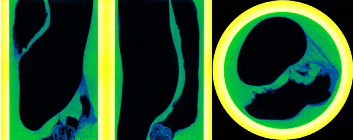
X-ray slices after hydrate formation. Color code: black= CO<sub>2</sub> gas; blue= hydrate; green= water saturated kaolin; yellow= aluminum chamber
