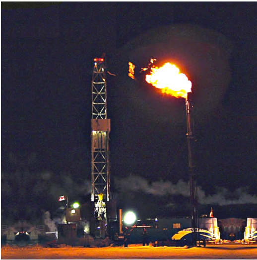
Fig I-3. Gas hydrates as a resource interest. (Left) Methane from hydrate flared from the Mallik 5L-38 Arctic gas hydrate research well in Canada (Courtesy of the Mallik 2002 Gas Hydrate Production Testing Program). (Right) Well-logging gas-hydrate-bearing sediment in the Gulf of Mexico (Courtesy R. Boswell, DOE).
