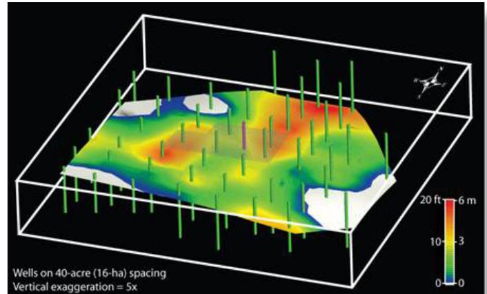
Depiction of reservoir model used for simulation of CO<sub>2</sub> flooding
