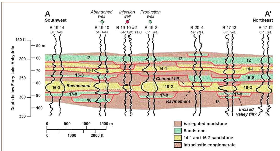
Cross-section through the pilot test area of the Citronelle Field shows the challenge of geologic complexity in fields where CO<sub>2</sub> flooding is being considered. Well B-19-10 #2 is the CO<sub>2</sub> injection well.
