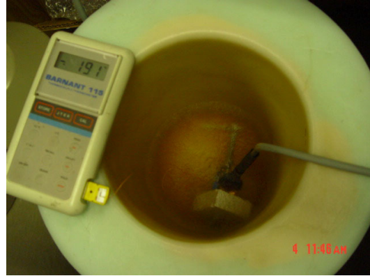
Fig. 7. Styrofoam and a C-clamp securing the sample to the Hot Disk sensor with entire assembly submerged into a liquid nitrogen bath.
