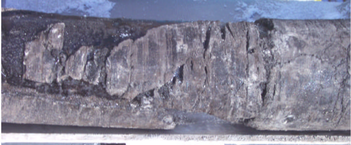
Figure 5. Another view of core shown in Figure 4 showing brecciation of the coal by the injection and freezing process that forms ice veins in Hot Ice Well, 650-654 ft TVD. Note brownish-black coloration of the coal typical of low rank coal. When in gauge, core diameter is about 3.4 inches.
