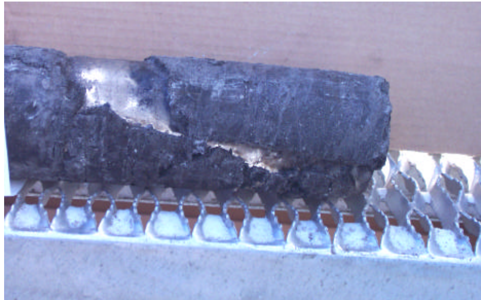
Figure 4. Ice vein cross-cutting coal, Anadarko Hot Ice #1 Well, 650-654 ft TVD. When in gauge, core diameter is about 3.4 inches.
