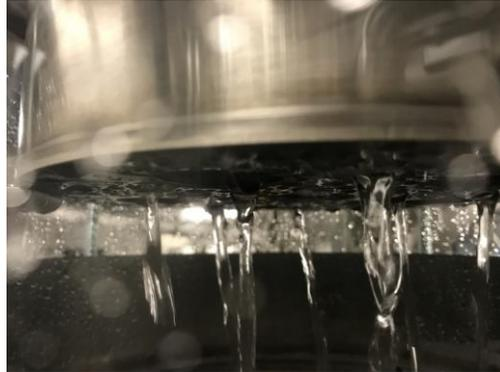
Top of 3D printed column packing
