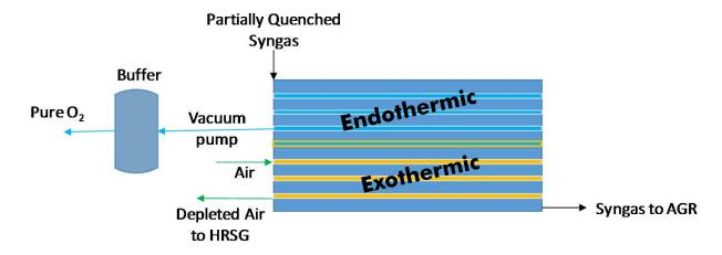
Process gas is used to maintain temperature
