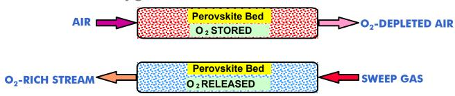
Between 2005 and 2008, under two separate Cooperative Agreements, a two-bed, 60-pph unit was developed by BOC/Linde and tested at WRI. The unit was integrated with an existing 250,000 Btu/h Combustion Test Facility to demonstrate oxy-fuel combustion concepts.
