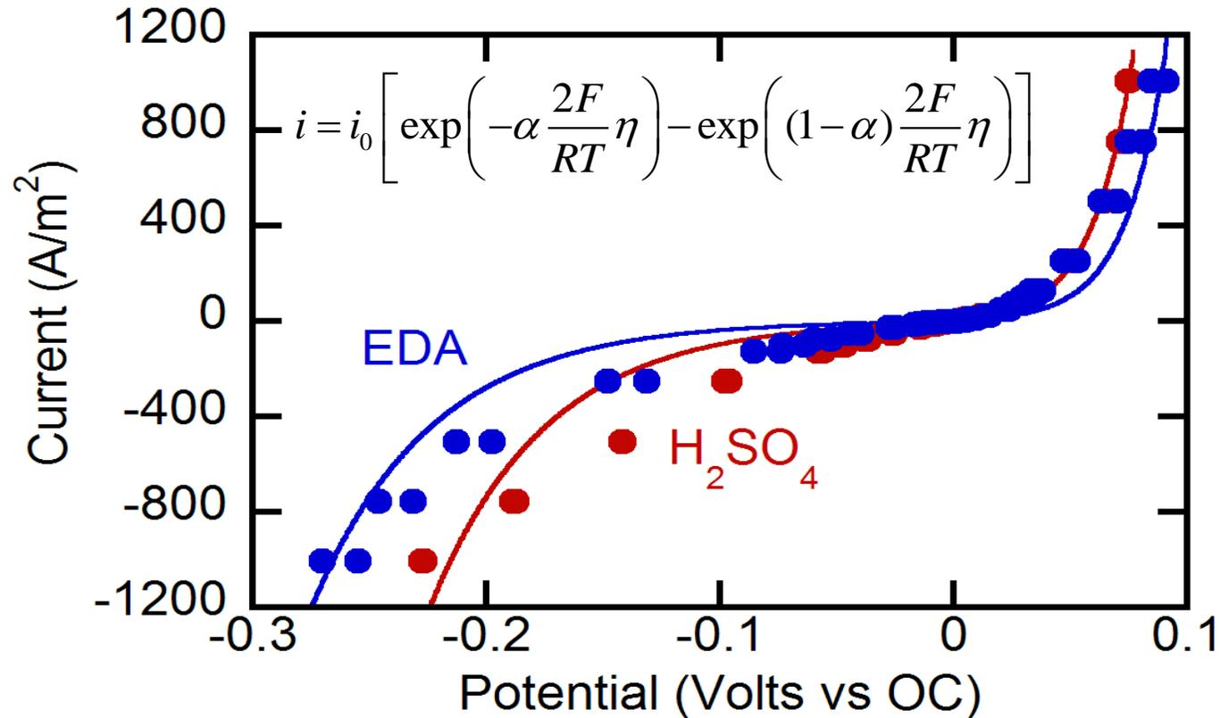
In absence of CO<sub>2</sub>, formation of EDA complex does not significantly hinder Cu deposition and dissolution. EDA Stabilizes Cu<sup>2+</sup> in solution
