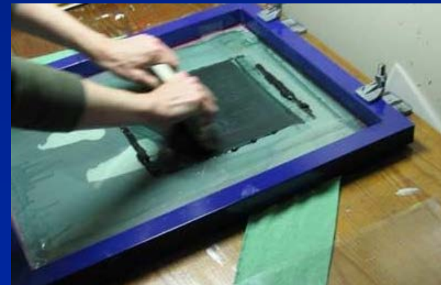
Screen printing for Applying the Contact Layer
