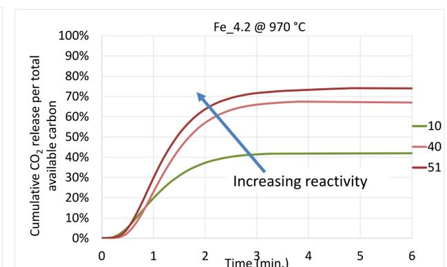
↑ Fe-based carrier under coal injection
