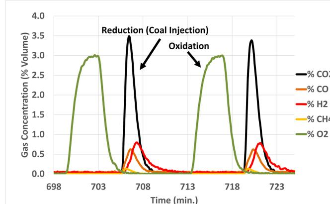
➤ CLC reaction commenced quickly as CO and CO<sub>2</sub> is formed immediately upon injection of lignite coal. Formation of CO<sub>2</sub> confirms CLC reaction, as no oxygen was fed to the reactor.
