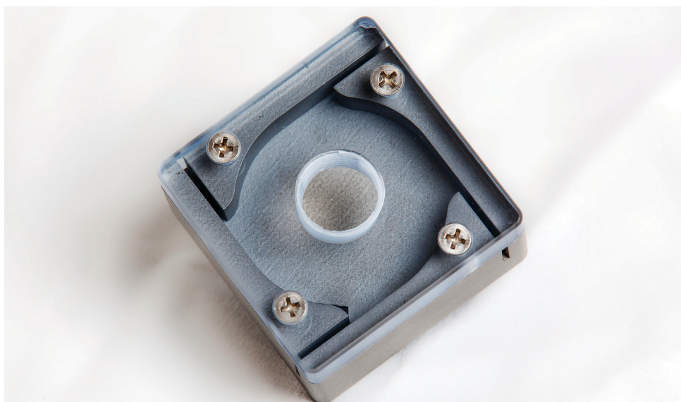
The successful simulations of the vortex chamber resulted in a prototype being manufactured through 3D printing for use in a bench-scale reactor.
