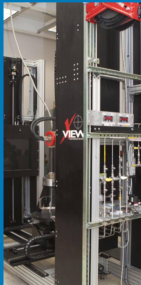
The industrial CT scanner can observe how fluid travels through rock core samples—giving researchers a glimpse of how CO 2 will react far underground.
