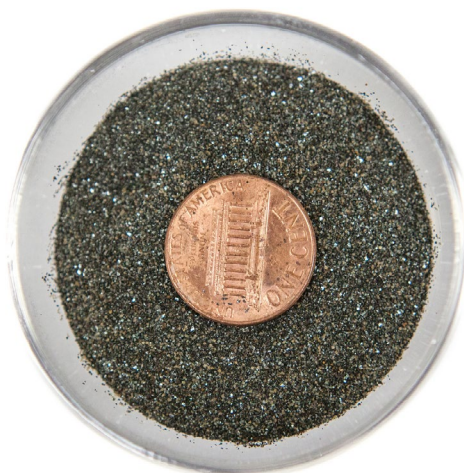
Oxygen carriers are similar in texture to sand. NETL researchers Drs. Ranjani Siriwardane and Duane Miller invented the oxygen carrier pictured here, which blends magnesium oxide and hematite.
